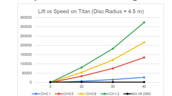
Fig. 4: Lift vs Speed on Titan. Graph created by M.Nosov using Excel, 2026.
