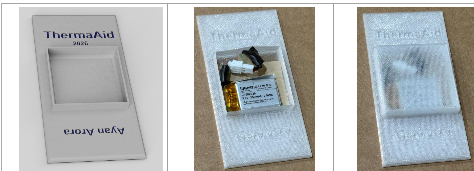
Figure 4: From 3D model to assembled ThermaAid active thermal matrix. The bio-safe TPU enclosure houses the electronics components demonstrating the low-profile, wearable form factor constraint.
